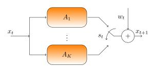
Markov jump linear systems are suitable in modeling dynamical systems with abrupt changes.
