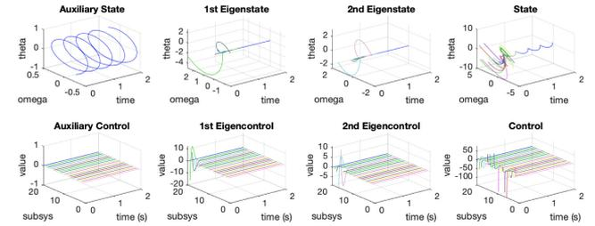
Fig. 5. Numerical example with Laplacian matrix coupling under the proposed optimal control on a network of 20 coupled harmonic oscillators over the time horizon  $T = 2$ .
